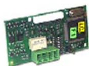
Fig. 11: Serial card for connection to a building management system
